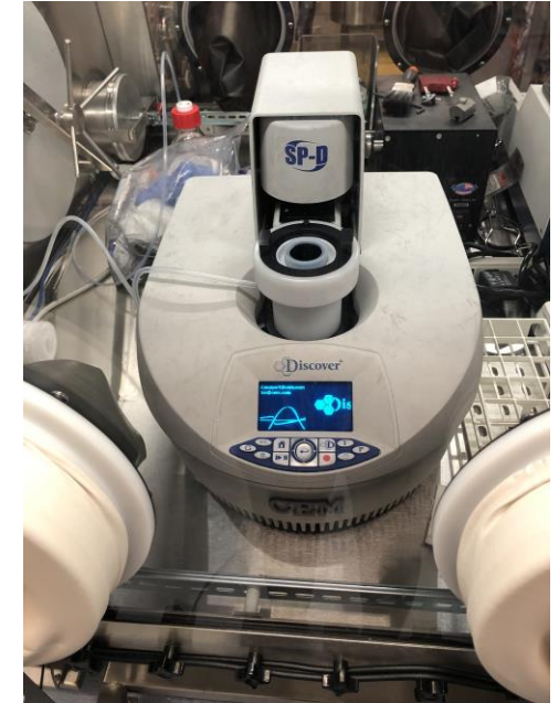
CEM Microwave digester in the glovebox train. The digester will help correlate redox measurements to elemental analysis of salt samples from the loop
