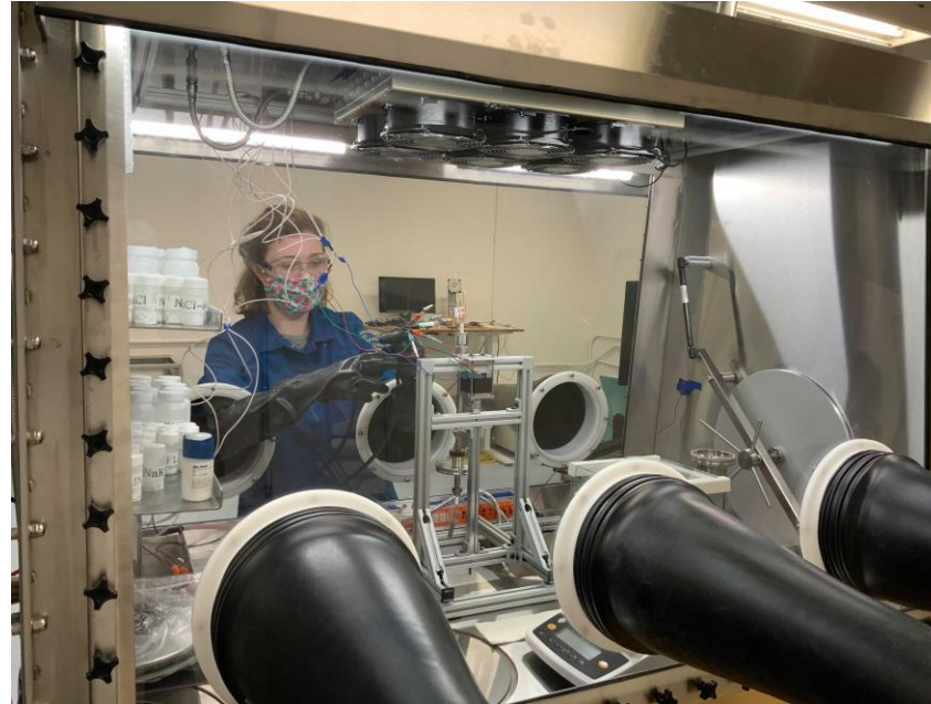
Commissioned glovebox train for experiments with irradiated materials and beryllium containing salts. The train is equipped with a deep well and an oil-free pump, which can be helpful for hydrogen and tritium experiments.
